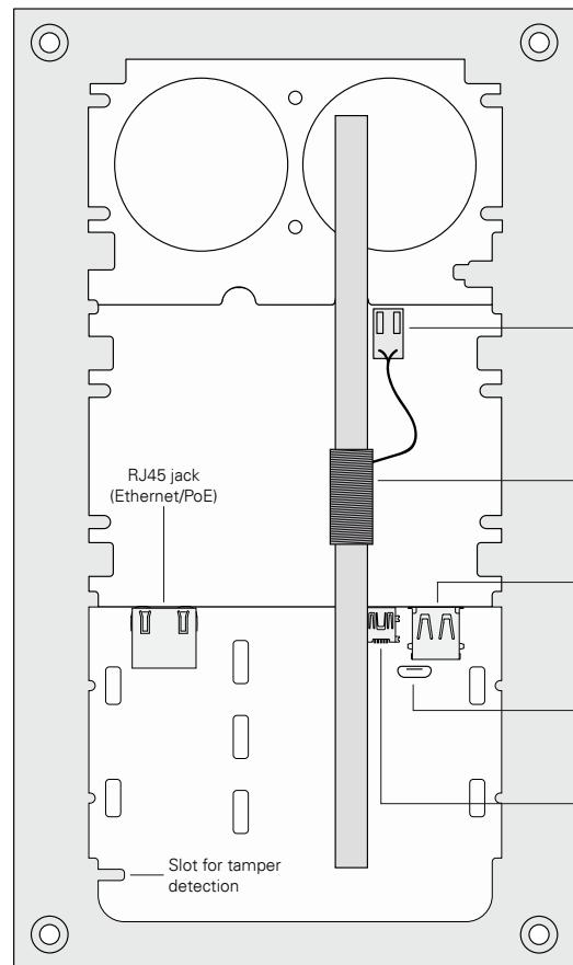
Install the tamper detection plate (for triggering the tamper detection alarm; in extent of supply) into the flush or surface mount box as shown in the following assembly drawing.
