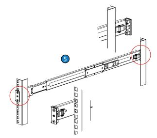
Output the slide rails to the frame of the rack. Attach the ends to the frame and press the bracket to fix the rail onto the frame.
